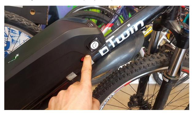
Turn on ebike display. If it doesn't turn of, try the battery rocker-switch in the other position.
