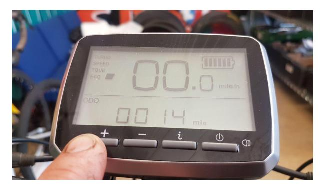
Press power button breifly, to activate the bike lights and / or illuminate the display.
