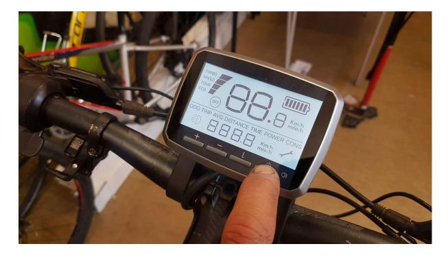
Use the "Plus" button to set power level to 'SPEED' ( recommended minimum for hill-climbing ).
